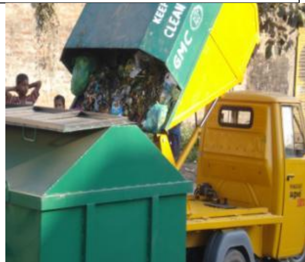
Photo showing how compatible equipments reduce manual handling of waste in Guwahati
