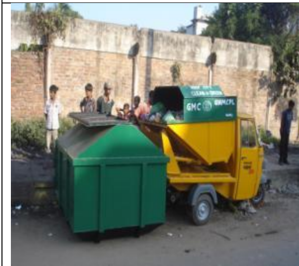
Photo showing how compatible equipments reduce manual handling of waste in Guwahati
