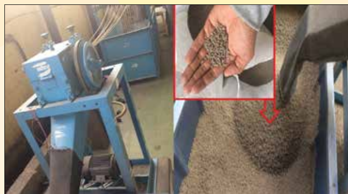
Figure 3.28 Various stages from plastic shredding to pellet making
